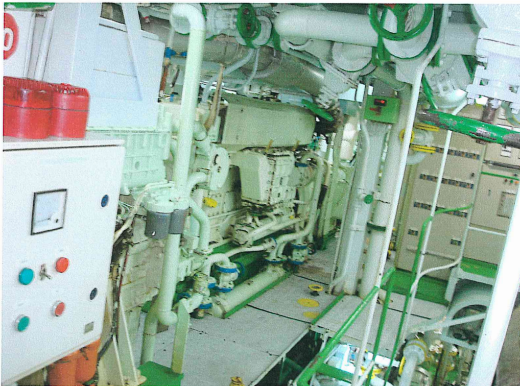
Port side Stork auxiliary engine
