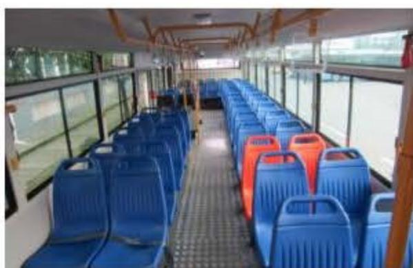
2+2 seat arrangement, with front door, middle door for disabled lift machine and rear door behind rear tire
