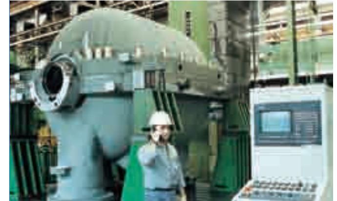
2MCL Horizontally split compressor being machined
