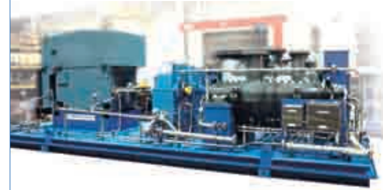
Horizontally split VS compressor for refrigeration service
