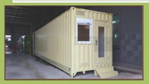
Size: L12192\*W2438\*H2896mm Structure : Modified 40ft HQ shipping container , 100mm thick rock wool sandwich panel decoration and insulation for wall ,roof and floor Configurations : kitchen , 4 pieces cabinets , bathroom fully fixtures, electrical and water plumbing Transport : Shipped as 40ft ISO shipping container
