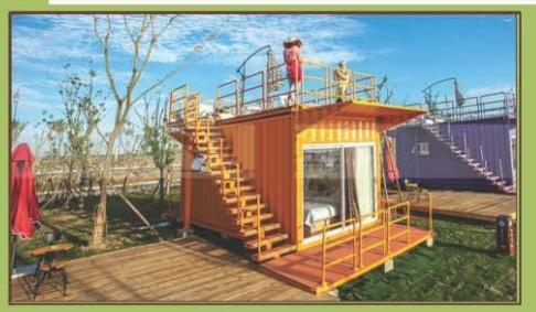
Size: L6058\*W2438\*H2591mm Structure : Modified 20ft ISO shipping container , 50mm fiberglass sandwich panel decoration Configurations : Roof platform , stair ,deck ,rain canopy,air conditioner ,wardrobe , table , bed , water heater ,bathroom fixtures and electrical Transport Shipped as 20ft ISO shipping container , roof platform ,stair ,decks and canopy will load inside extra container for shipping FOB price : 22500 USD
