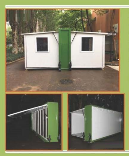
Opening size: L5800\* W5184\* H2500mm Closing size :L5800\*W700\*H2500mm Structure : steel structure + sandwich panel + insulation , 3 people 10 minutes can opening without crane Configurations : electricity ,gas strut ,lift wheels ,4 windows ,2 doors Transport : 1\*40ft HQ load 6 units
