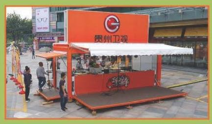
Size: L6058 x W2438 x H2591mm Structure : Modified ISO 20ft shipping container, sandwich panel decoration and insulation Configurations : automatic awning ,hydraulic system , electrical and water plumbing system Transport : Shipped as ISO 20ft GP shipping container
