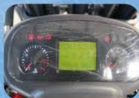
智能仪表盘 Combination Meter Necessary instrumentation, such as the fuel meter, water temperature indicator and hour meters are shown in an easy-to-monitor digital format.
