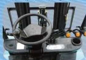
智能仪表盘 Combination Meter Necessary instrumentation, such as the fuel meter, water temperature indicator and hour meters are shown in an easy-to-monitor digital format.
