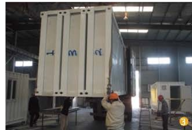
CONTAINER LOADING (1x40'HQ loads 6 sets of 5850mm Length Flat Packs with Rollers For Easy Roll In And Out into the Shipping Container)
