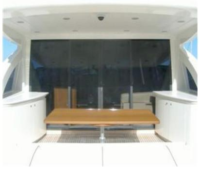
Garage with Hydraulic controlled opening hosting a 4,20 mt Tender boat (equipped with hydrojets)
