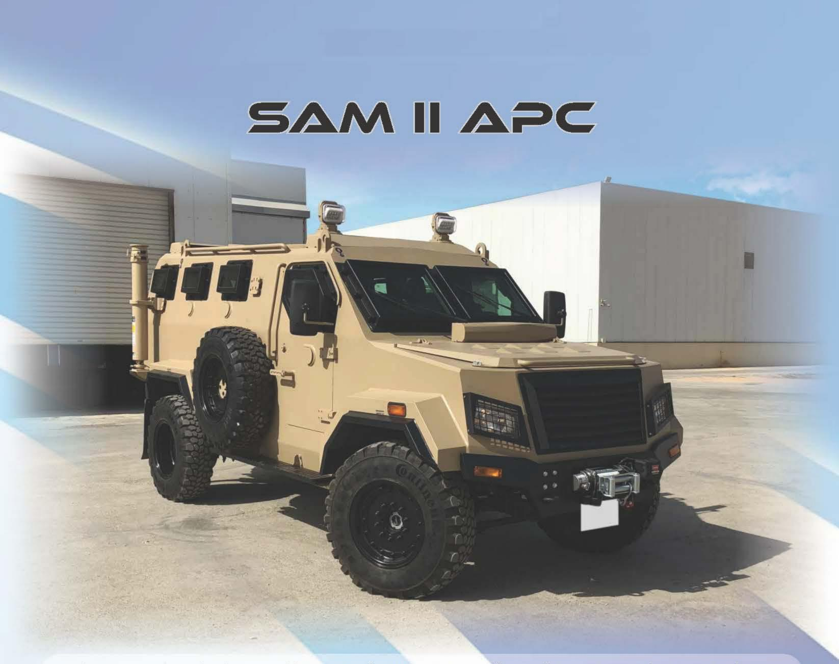
**SAM II APC** is the latest addition to the Rhino Defence fleet of ingenious solutions. Built monocoque using a Ford F-550 Super duty drive train with upgraded suspension. This unique approach makes SAM II cost effective yet capable to withstand greater threats and to compete with rivals.
