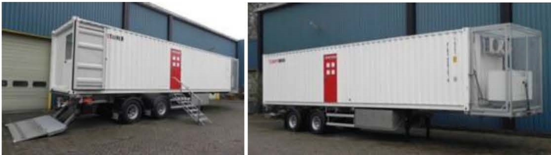
Trailer with hydraulic lift, stairs, water tanks, levelling legs and generator in rack at the front.
