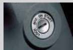
Double Locking System The basic feature deters theft and prevents accidental starting.
