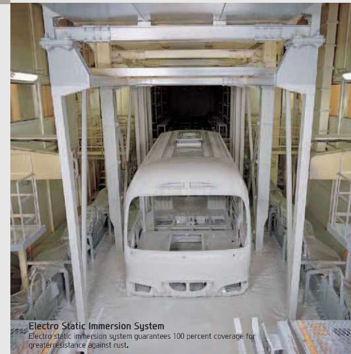
Engine Bay Electro static immersion system guarantees 100 percent coverage for greater resistance against rust.
