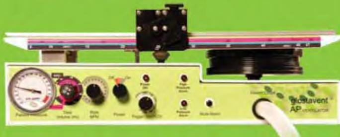
The ventilator is a time-cycled, volume limited, pressure generator. It consists of a set of gas driven bellows. The drive gas is oxygen at a pressure of 140 KPa supplied either by the concentrator or, in the event of an electricity failure, from the reserve oxygen cylinder or external oxygen source. After it has driven the ventilator it is collected and returned to the breathing circuit to supplement the inspired oxygen concentration, always providing the patient with a minimum of 35% oxygen.
