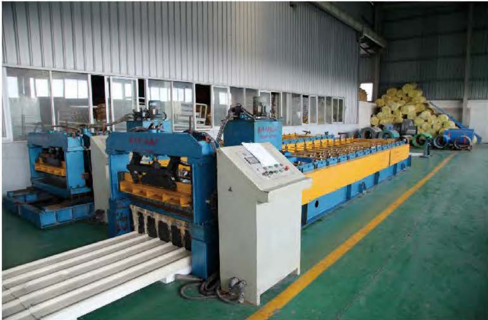
Roof panel production line
