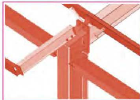
▲ Cornice Connection Point
