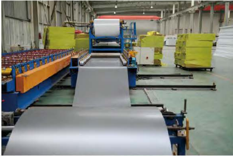
Sandwich panel production line
