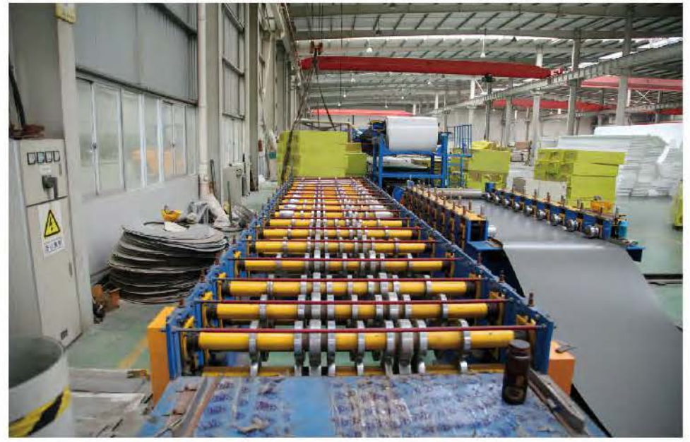
Sandwich panel production line
