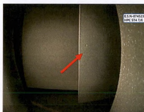
MINOR DENT ON T/E AIRFOIL
