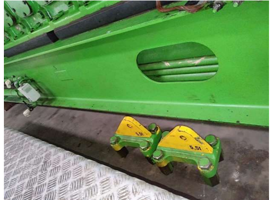
Engine lifting lug B-side
