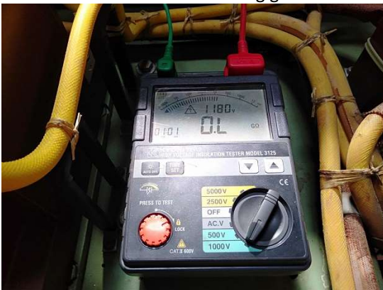
Phase V insulation resistance: >1 giga ohm
