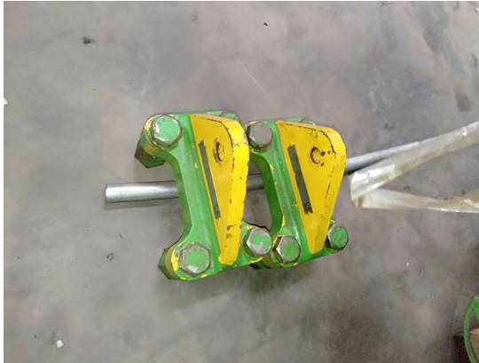
Engine lifting lug A-side
