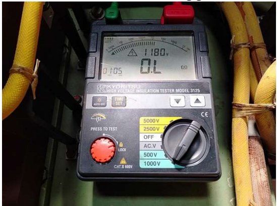
Phase U insulation resistance: >1 giga ohm
