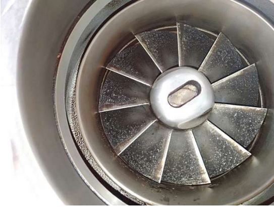
Bank A: Easy turn by hand (gab: 0,45mm)
