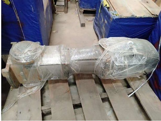
HT circuit circulation pump
