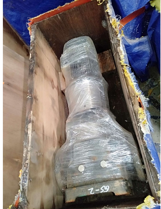
LT circuit circulation pump
