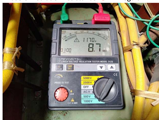
Phase U insulation resistance: 8.7 mega ohm
