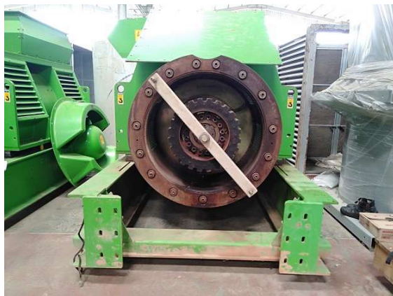
Generator rotor lock bar
