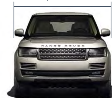
Obstacle Clearance Off-road height 296.1mm Standard ride height 221.1mm
