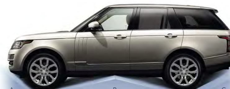
Obstacle Clearance Off-road height 296.1mm Standard ride height 221.1mm
