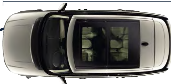
Standard Overall length 4,999mm (Long Wheelbase 5,199mm)
