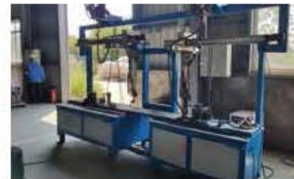
Roof Short Beam Automatic Welding Machine
