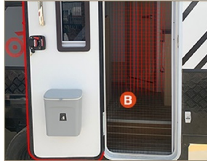
Installed with push-pull screen door.
