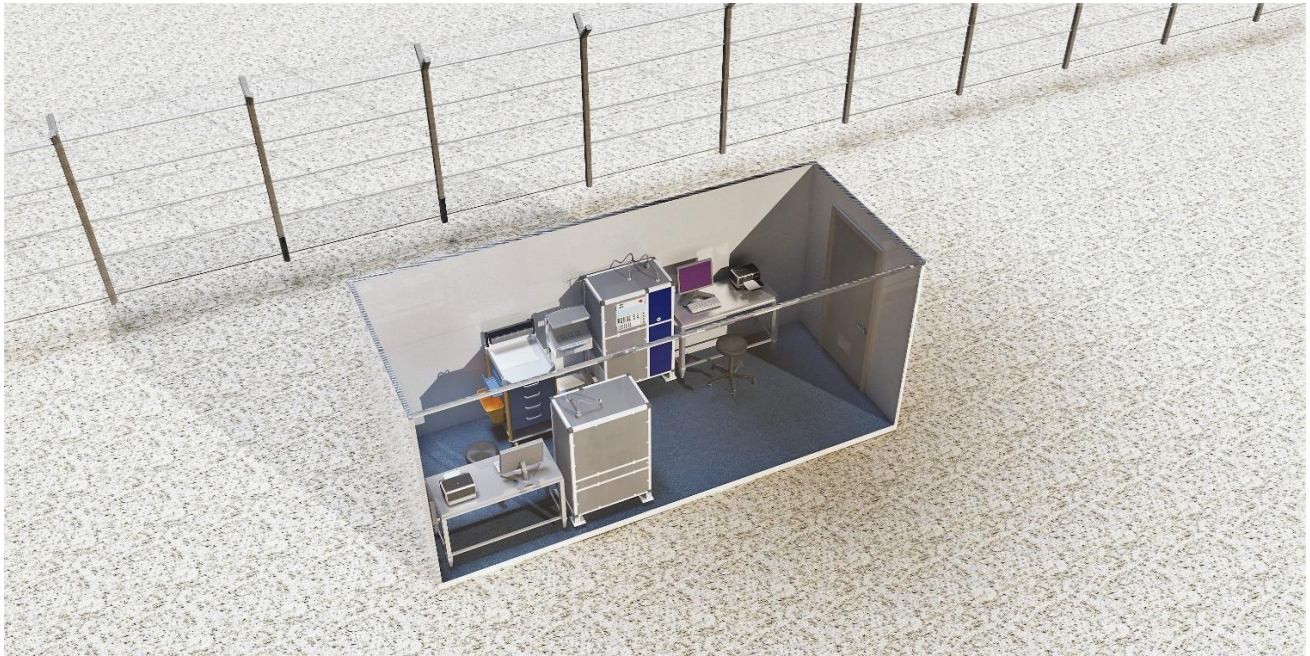
20 FT Container Design for Laboratory & Pharmacy Unit
