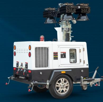
LED technology lighting towers is equipped with LED floodlights which guarantee optimal use of the battery and soalr system, The LED lights can be adjusted and rotation 360 degree manual for cover more area
