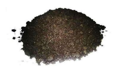
Product characteristics: OXI BRICKS is a substance composed mainly by Iron Oxide, Carbon and other
