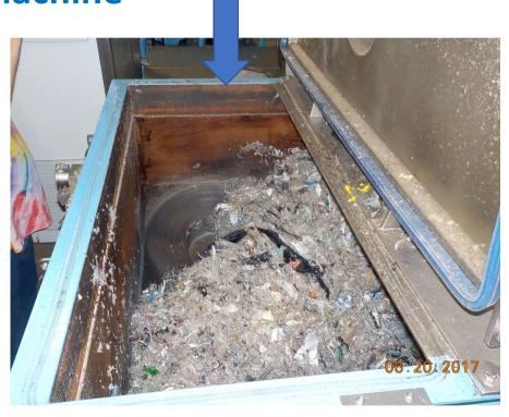
The waste is now dried so it no longer smells and is exiting the BCF mixer. It is no longer considered waste. It is renewable Reengineered Carbon Fuel.
