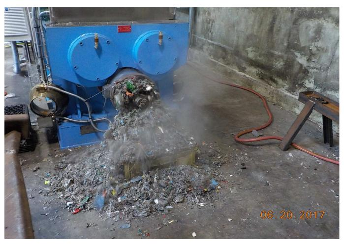
This Super RDF (Refused Derived Fuel) is now ready to be conveyed to the conversion systems that produce renewable diesel fuel, renewable jet fuel and or renewable Hydrogen from this dry carbon based feedstock.
