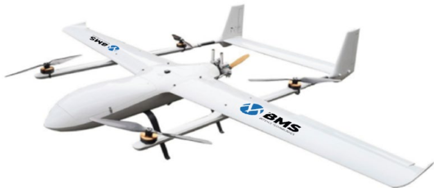
AEROGARD V3800 -H VTOL "AYBARS-1" (Hybrid, Electric + Liquid Fuel Engine, Payload 15 Kg.)
