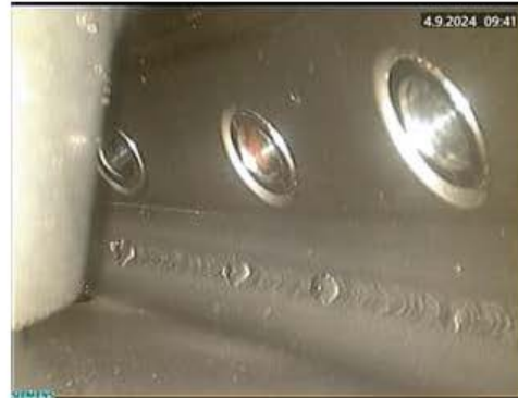
Burner #10 inner chanel with droplets of water
