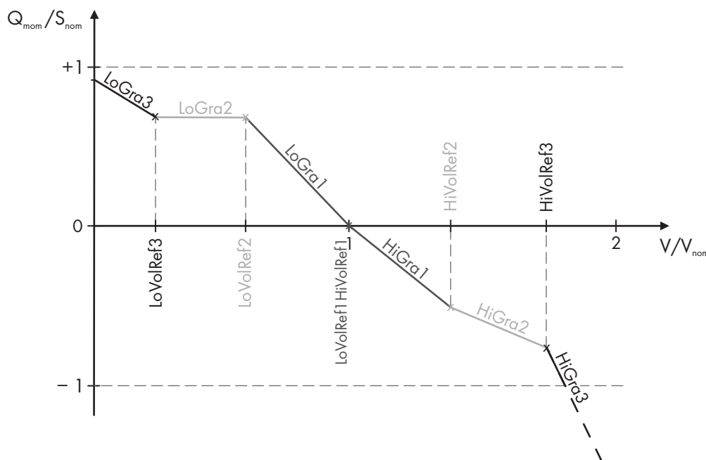
Figure 127: Characteristic curve of the voltage-dependent reactive power control
