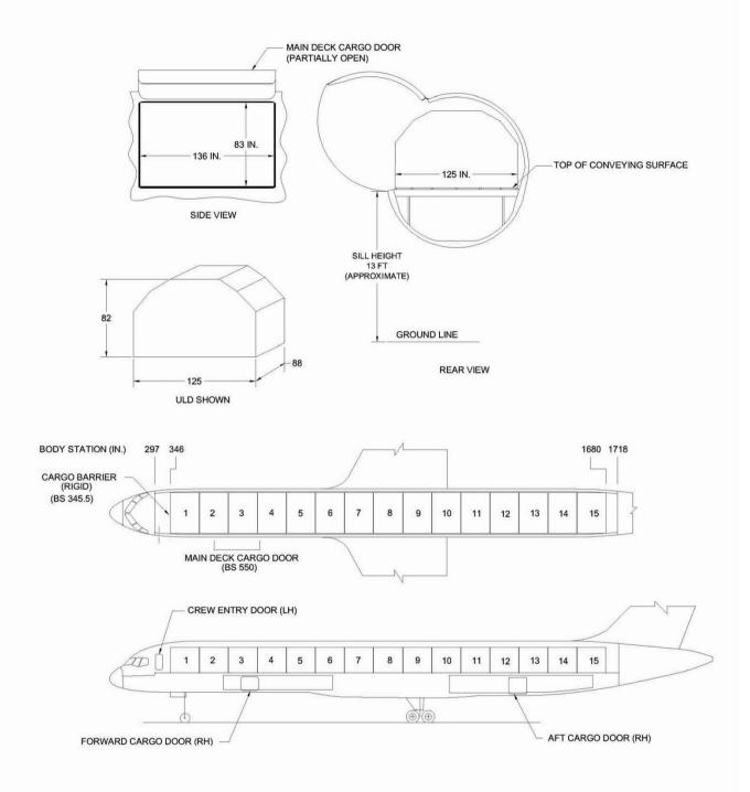
Figure 2.0-3: Interior Arrangement – Main Deck Cargo, 15 ULDs
