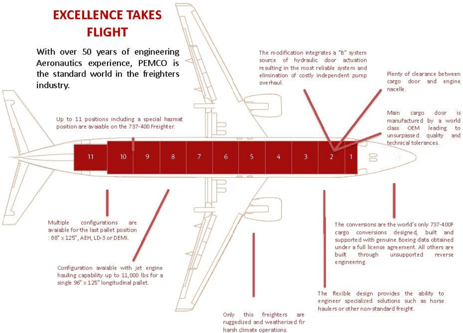
With its increased payload and volume capabilities, the 400F may be the most desirable sub-30 ton freighter yet. In response to increasing market demand, are two distinct options – A 11-position high yield freighter<sup>1</sup> and a full-freighter<sup>2</sup>.
