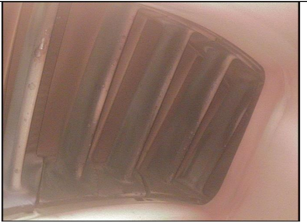
Picture 06: HP turbine nozzles & blades #7
