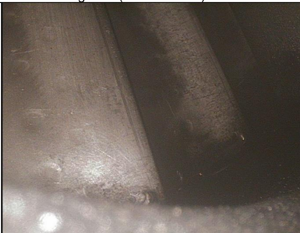
Picture 07: stg 1 IGV (to outer casing)
