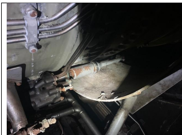
Picture 01: IGV compressor 6 o'clock corrosion
