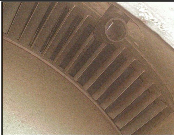
Picture 15: Pressure probe & OGV
