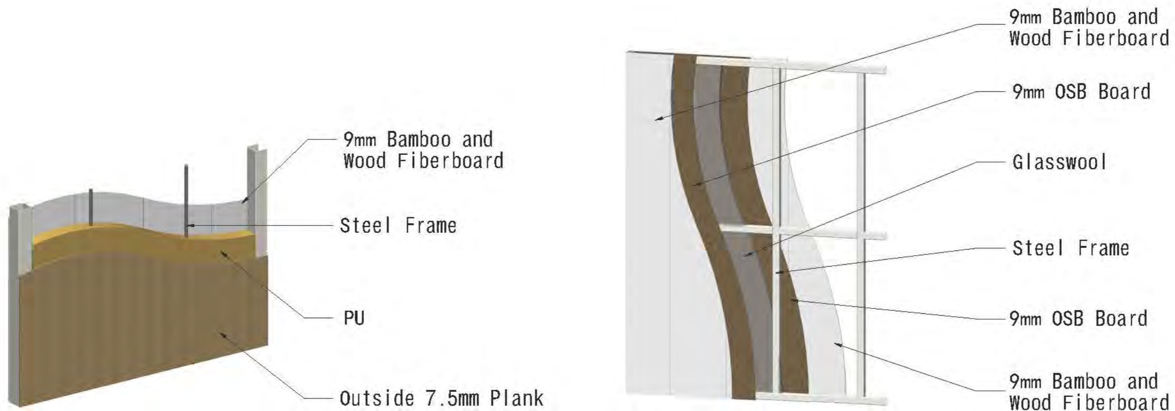
Section View of Interior Wallboard
