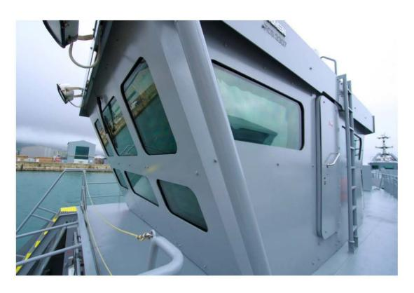
All around the wheelhouse, armoured plating is fitted.
