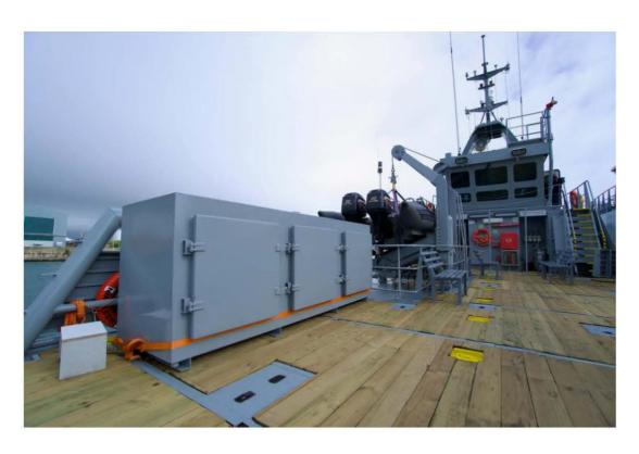
Deck lockers, on both SB and PS side, for storage purpose.
