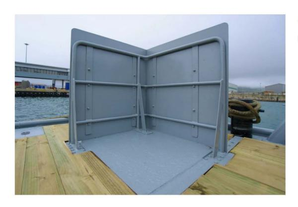
Situated on the aft deck on both PS and SB, armoured protection by means of steel plating.
