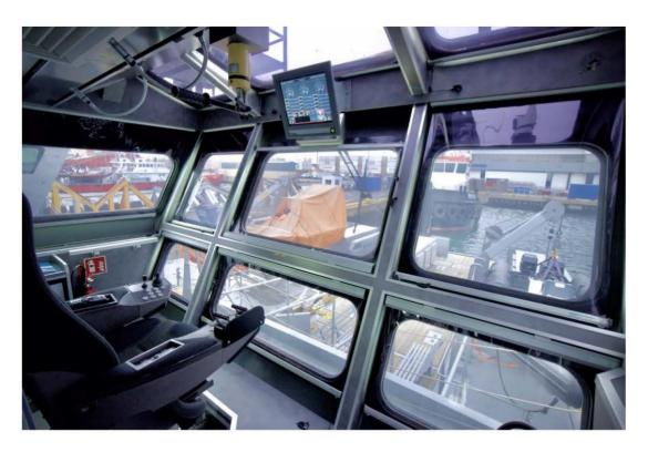
The captain can operate the vessel also from this aft position.
