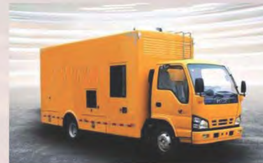
Emergency power supply vehicle
