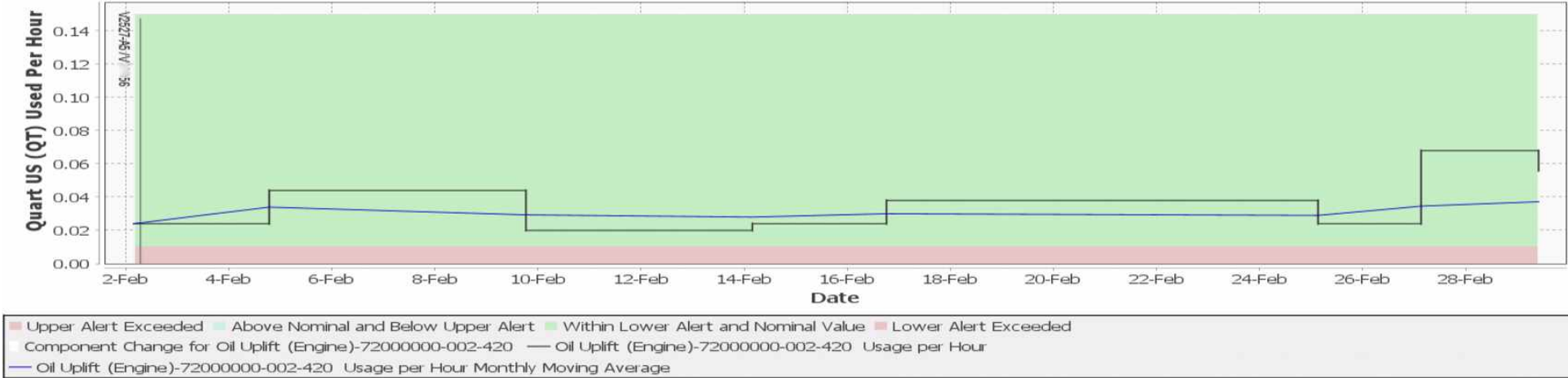
Analysis For Oil Uplift (Engine) for ENGINE - ASSY V2500 at Pos 002,Zone 420
