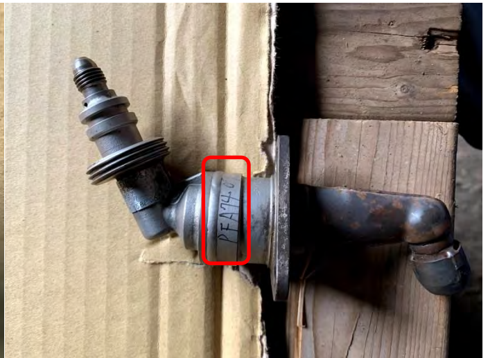
Fuel nozzle clean and Serial Number
