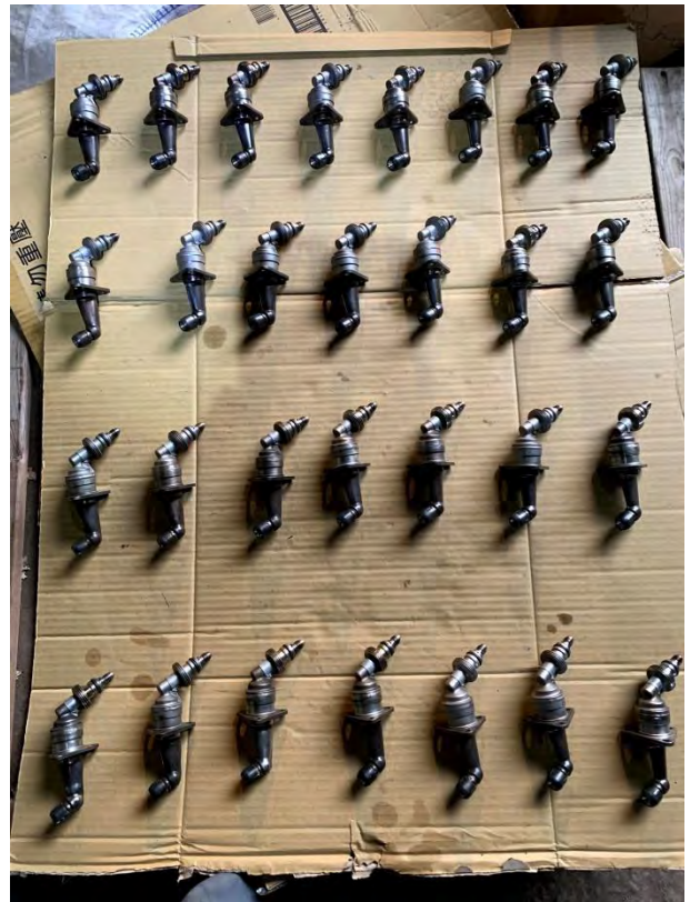
Fuel nozzle clean and Serial Number
