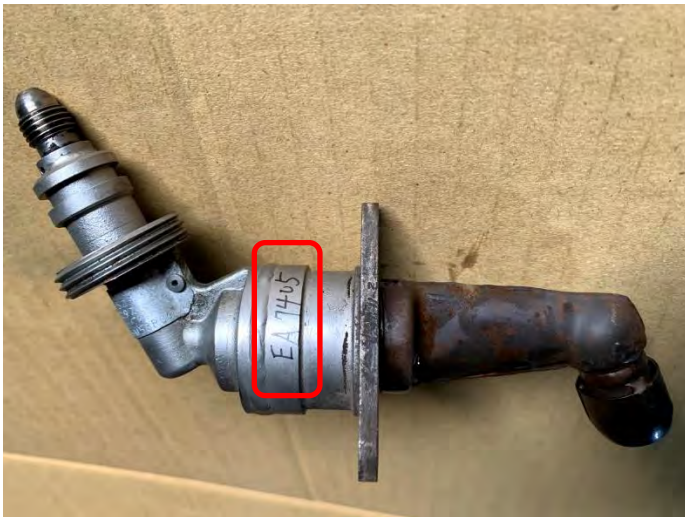
Fuel nozzle clean and Serial Number
