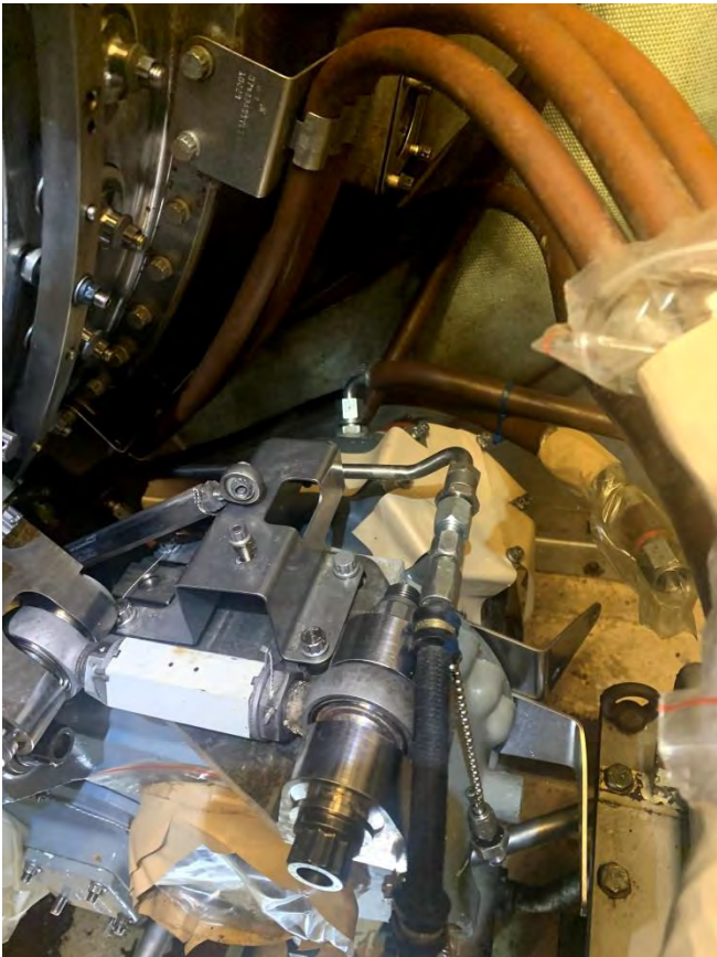
A- Sump-#3 Bearing And accessory gearbox(CFF)
