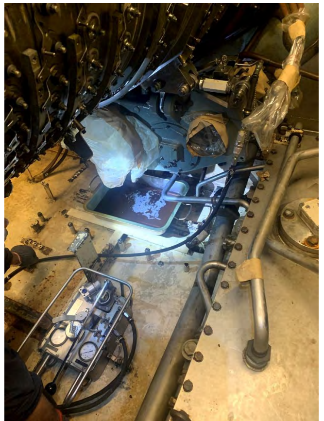
A- Sump-#3 Bearing And accessory gearbox(CFF)
