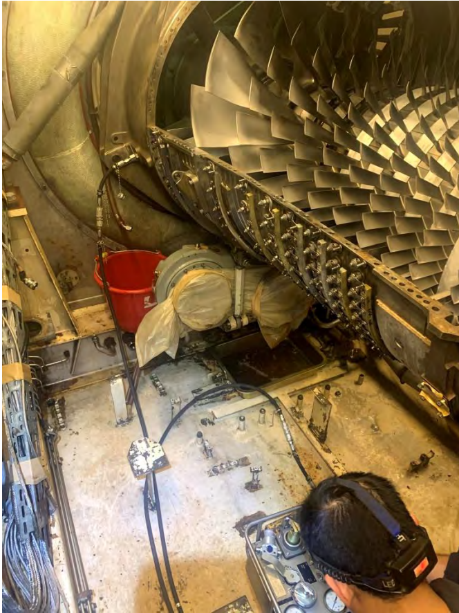
A- Sump-#3 Bearing And accessory gearbox(CFF)
