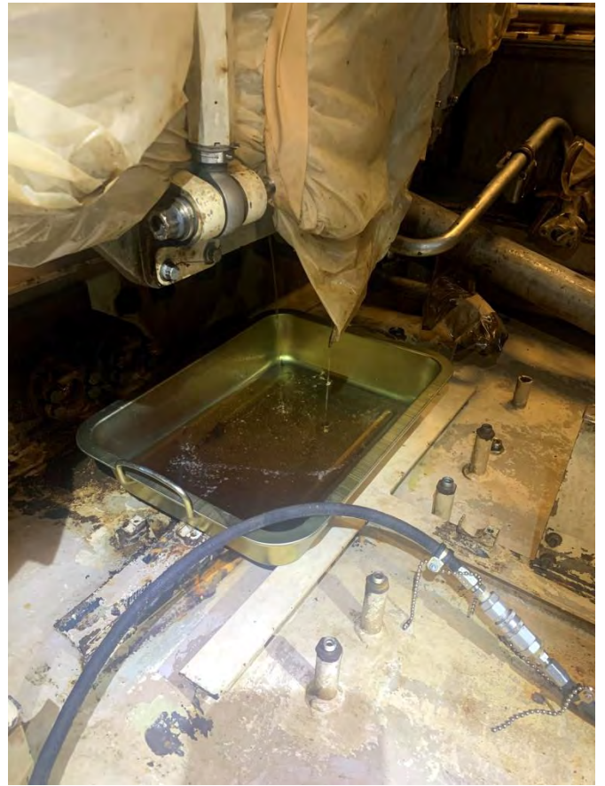
A- Sump-#3 Bearing And accessory gearbox(CFF)
