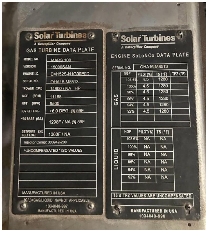
The technical characteristics of the turbines are shown in the attached table.
