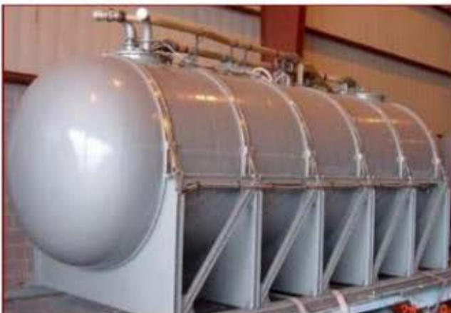
Includes the 3600 Gallon Fuselage Fuel Tank
