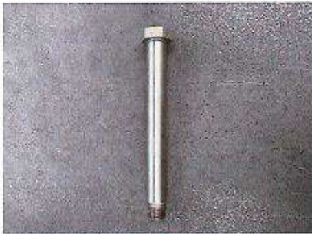
TOW FITTING BOLT - O/DIAMETER UNDERSIZE
