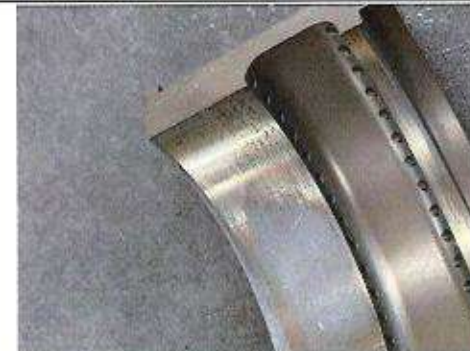
UPPER BEARING – WORN
