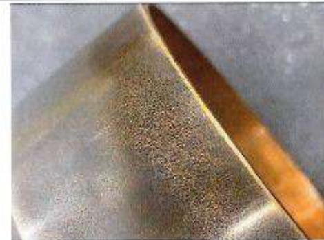
INSERT – COATING WORN THROUGH
